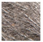
**Fibrais 300** is a shaped product, obtained with threads of normal titles, cut to a length of 50 mm bonded together by a binder emulsion, soluble styrene and compatible with polyester resins.
