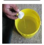
**Fiais** is a liquid additive in mineral base with high concentration that because of its exotermic reaction is able to decrises the freeze point of mixwater and increases the hydratation of the cement allowing the concreting at low temperatures. (UNE-EN 934-2 and 3)
