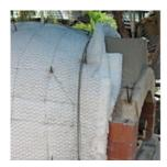
The ceramic fiber modules are produced by a compressed ceramic cover. Specially developed to improve the thermal insulation of industrial furnaces and other applications.
