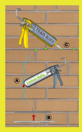
For a proper refurbishment on facades made of face bricks is necessary to combine the various reparation processes of this brochure according with the type of fissure or crack being on the facade.
